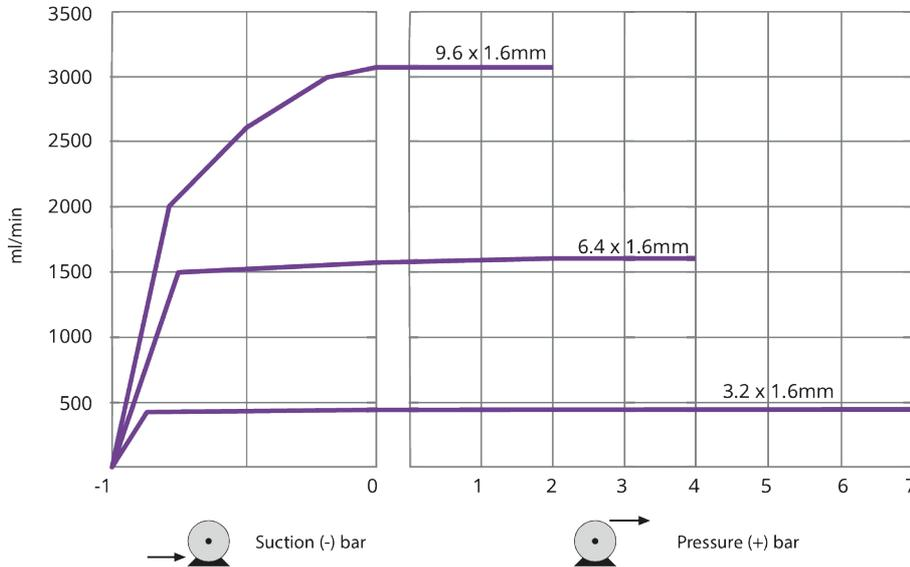
To achieve the discharge pressures stated above, the rotor must be run counter clockwise. To achieve optimal tube life, run the rotor clockwise at a maximum discharge pressure of 2 bar.
