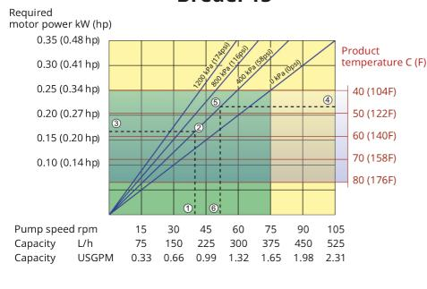
Note: The area of continuous operation diminishes with increased product temperatures. For product temperatures >40C, the area of continuous operation reduces to the corresponding red
