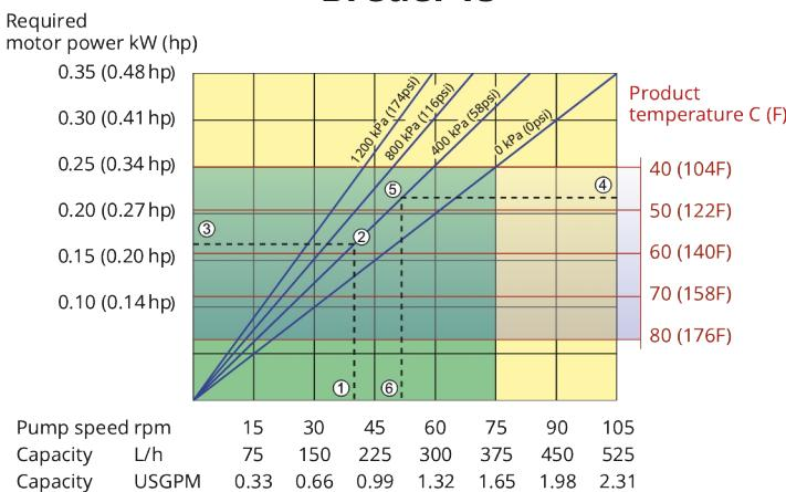
Note: The area of continuous operation diminishes with increased product temperatures. For product temperatures >40°C, the area of continuous operation reduces to the corresponding red temperature line.
