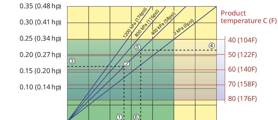
Note: The area of continuous operation diminishes with increased product temperatures. For product temperatures >40C, the area of continuous operation reduces to the corresponding red temperature line.
