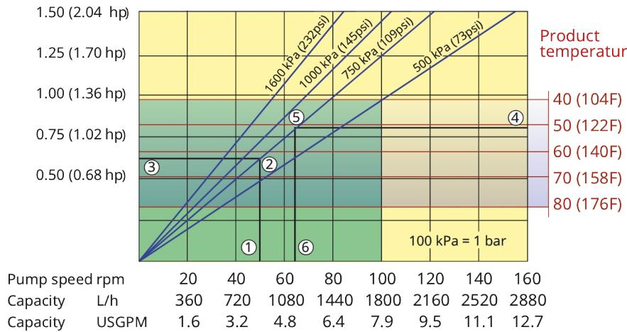
Note: The area of continuous operation diminishes with increased product temperatures. For product temperatures >40°C, the area of continuous operation reduces to the corresponding red temperature line.
