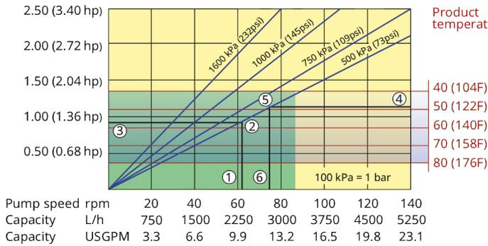
Note: The area of continuous operation diminishes with increased product temperatures. For product temperatures >40C, the area of continuous operation reduces to the corresponding red temperature line.
