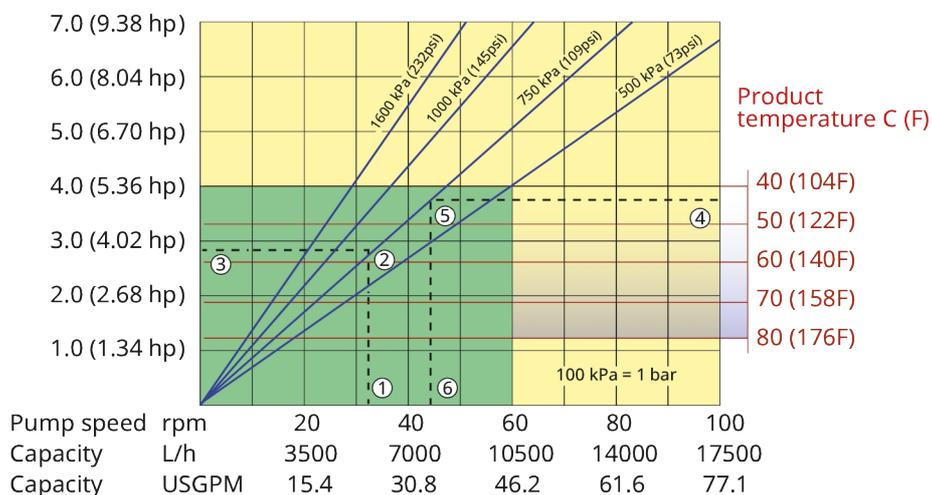
1. Flow required indicates pump speed
