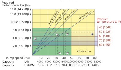
Note: The area of continuous operation diminishes with increased product temperatures. For product temperatures >40C, the area of continuous operation reduces to the corresponding red temperature line.
