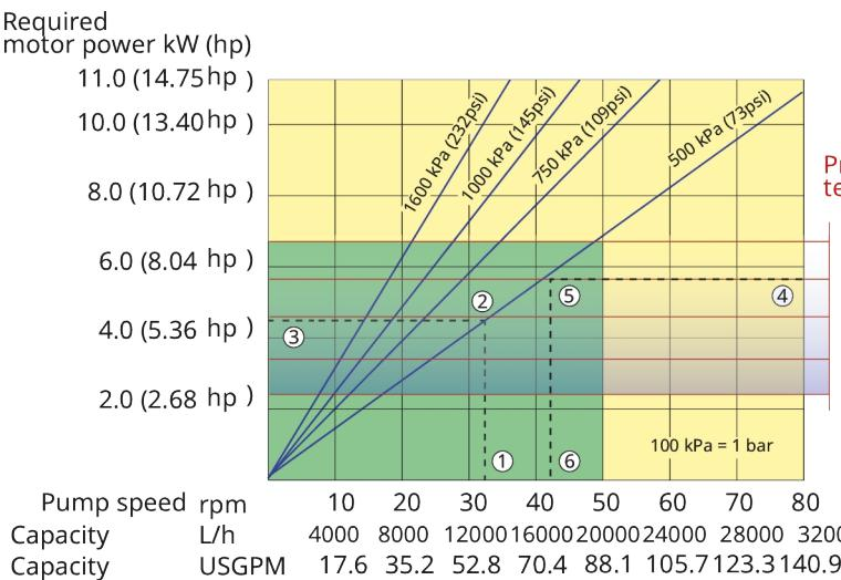
Note: The area of continuous operation diminishes with increased product temperatures. For product temperatures >40C, the area of continuous operation reduces to the corresponding red temperature line.
