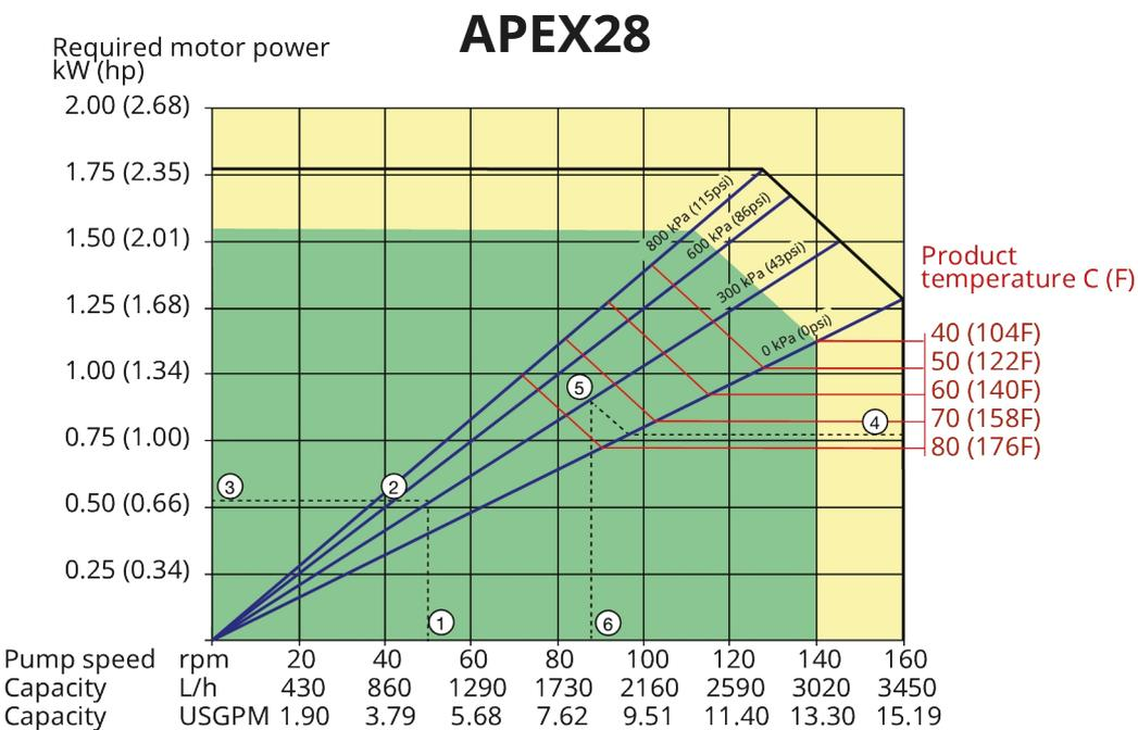
1. Flow required indicates pump speed
