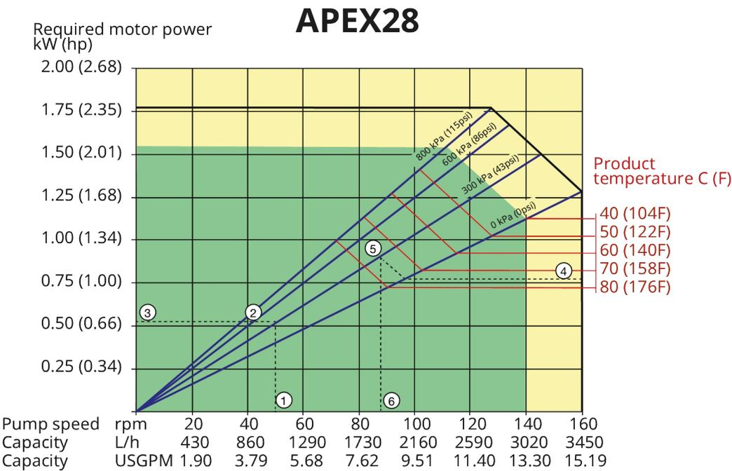
1. Flow required indicates pump speed
