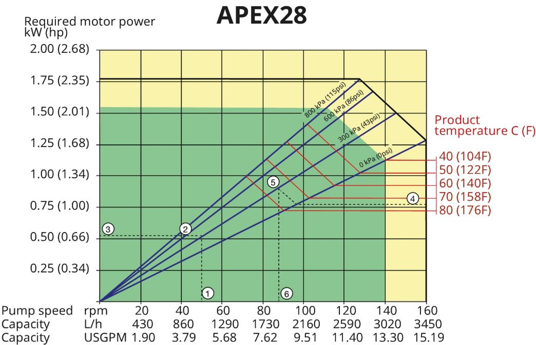
1. Flow required indicates pump speed
