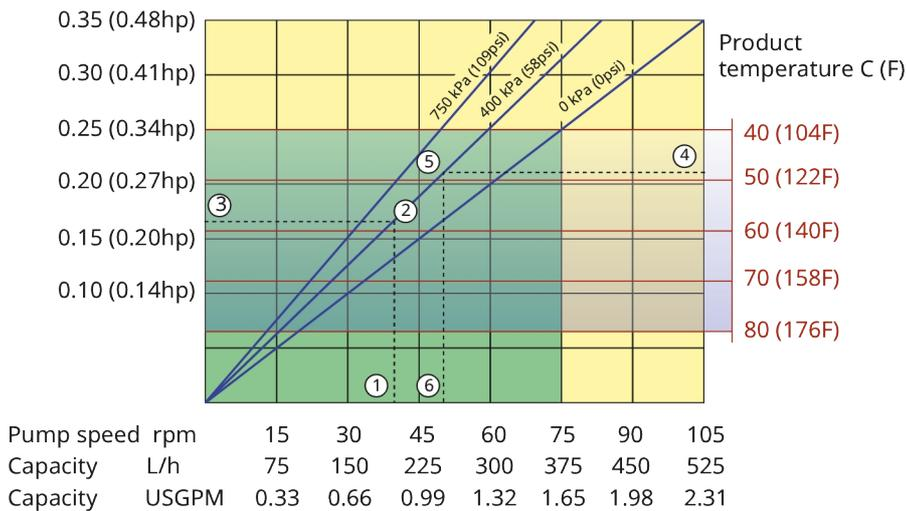
1. Flow required indicates pump speed
