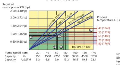
Note: The area of continuous operation diminishes with increased product temperatures. For product temperatures >40C, the area of continuous operation reduces to the corresponding red temperature line.
