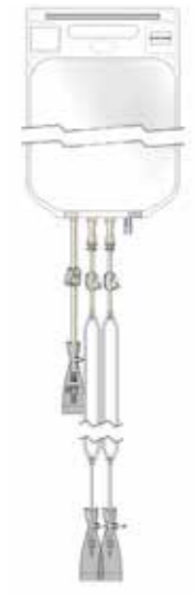
Configuration C Accusil tubing, MPC connector and 2 PEI filling nozzles The distance between the filling nozzle and the Y-connector is 30cm The distance between the Y-connector and the bag is 150cm The inlet tubing has a length of 30cm
