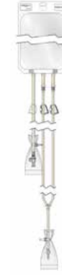
Configuration B Accusil tubing, MPC connector and PEI filling nozzle The distance between the filling nozzle and the Y-connector is 30cm The distance between the Y-connector and the bag is 150cm The inlet tubing has a length of 30cm
