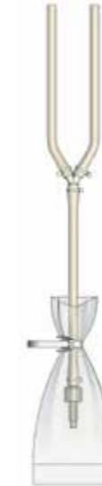
Configuration A Accusil tubing and PEI nozzle The distance between the filling nozzle and the Y-connector is 30cm There are two lengths of tubing after the Y-connector, each with a length of 210cm
