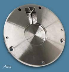
Certa front housing before and after re-machining to restore Certa's performance back to original factory specification.
