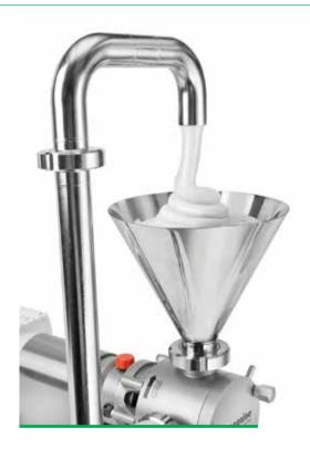
Put simply, if a production or process plant changes to a higher viscosity product, the impact on a sine pump is minimal is not negligible. For instance, using the same application parameters as before, but switching from a 20,000cP product to a 200,000cP product, the VHP of a sine pump increases by around 0.1, to 0.3VHP (0.22kW).
