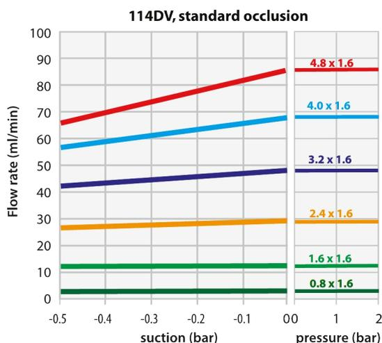
Flows obtained pumping water at 100rpm CCW-rotation
