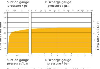
Flow rates based on pumping water at 20C with zero suction and delivery heads
