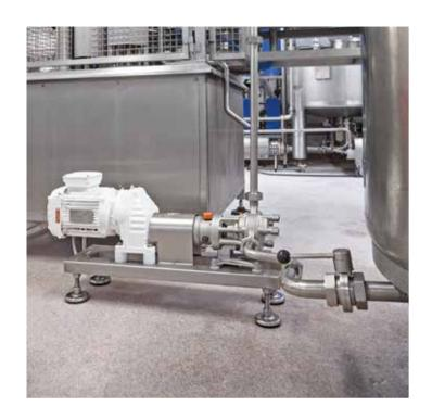
Certa by MasoSine outperforms lobe pumps in critical food and beverage applications. The sinusoidal rotor design of our MasoSine pumps delivers a lower shear, gentle pumping action that safely transfers delicate food products without risk of degradation.
